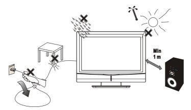
Ensure that the TV placed in a position to allow free flow of air. Do not cover the ventilation openings on the back cover.
